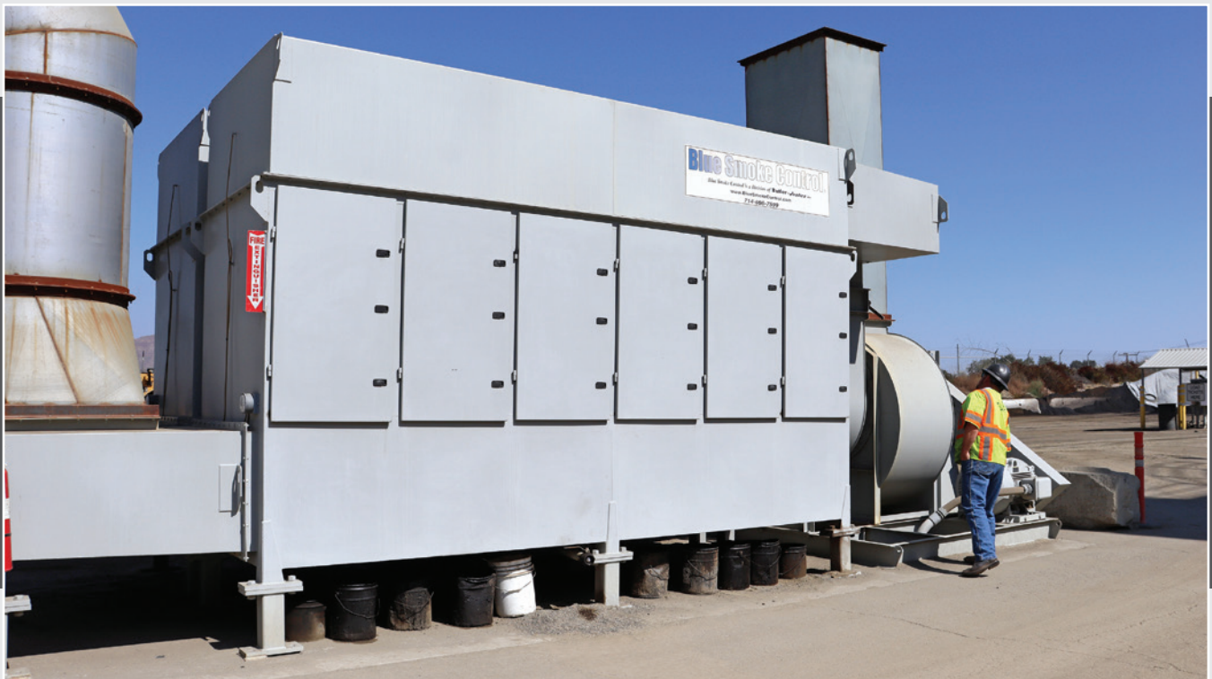
Above: Blue Smoke Control from Butler-Justice, Inc. captures blue smoke from key emission points in the asphalt production process
