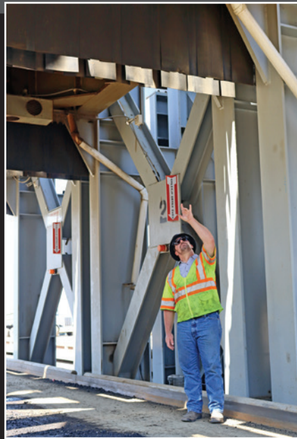
Above Left: Todd Fields, Butler-Justice, Inc., points to the gates below the silos that are vented with a damper control collection system from Butler-Justice, Inc.
